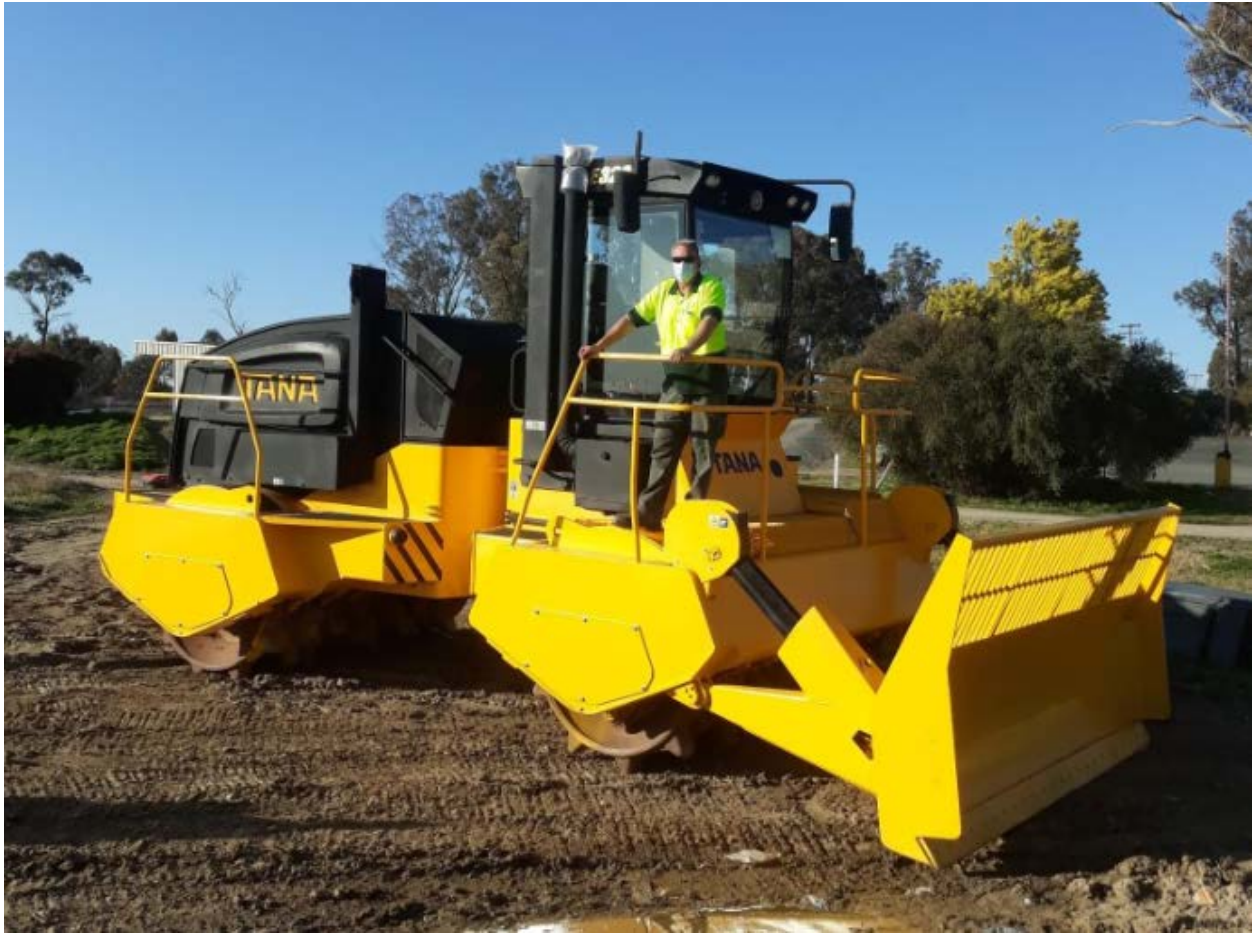
Figure 2 – Landfill Compactor (acquired 1 September 2021)
