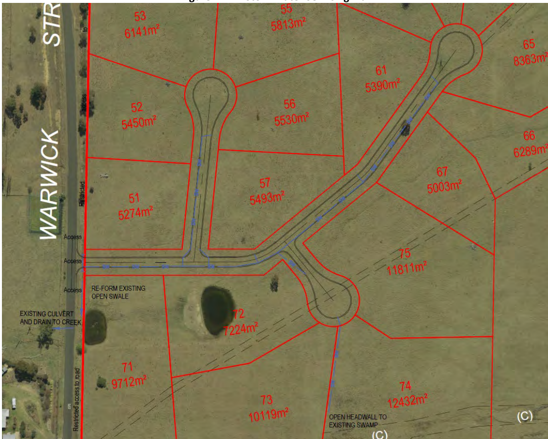
Figure 17.7B Stormwater Servicing Plan
