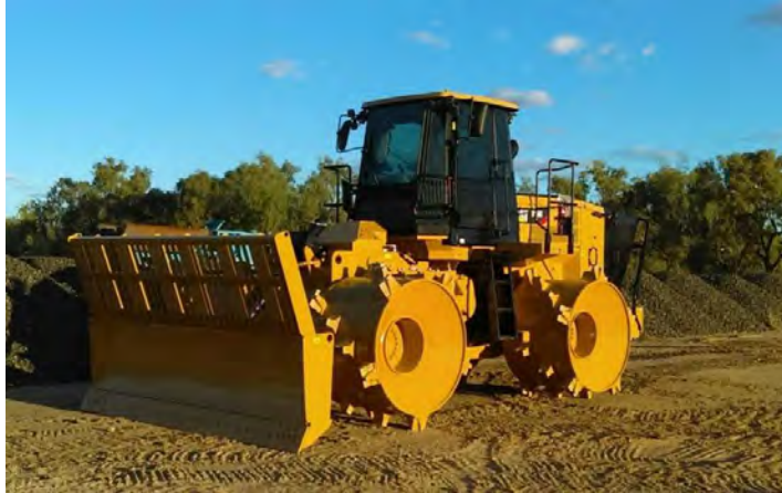
Figure 3-2 Caterpillar 816K Waste Compactor
