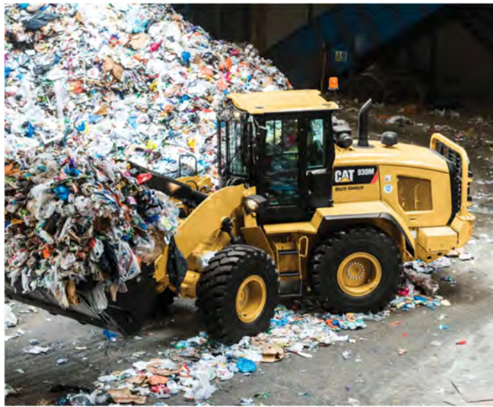
Figure 3-1 Caterpillar 930M Wheel Loader with Waste Handler Accessories
