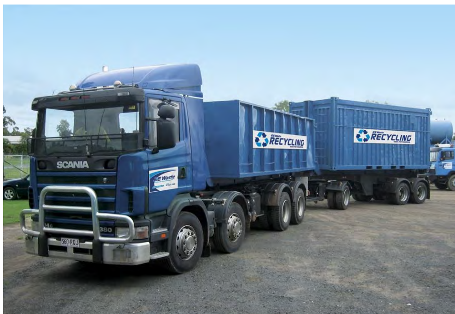
Figure 3-5 Hook-Lift truck hauling two skips with dog trailer
