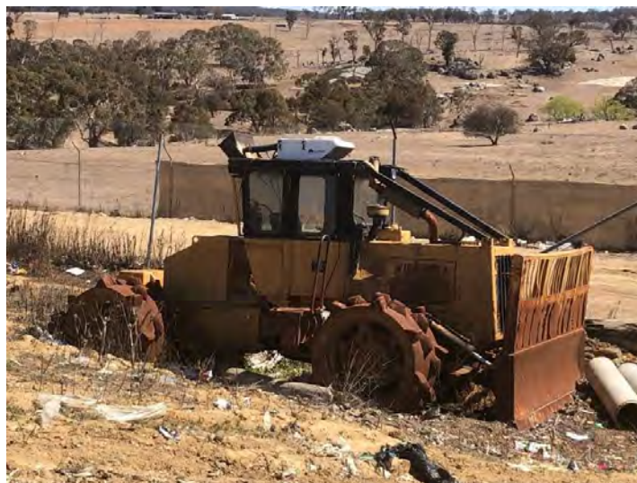
Figure 2-8 USC Waste Compactor (Out of Order)
