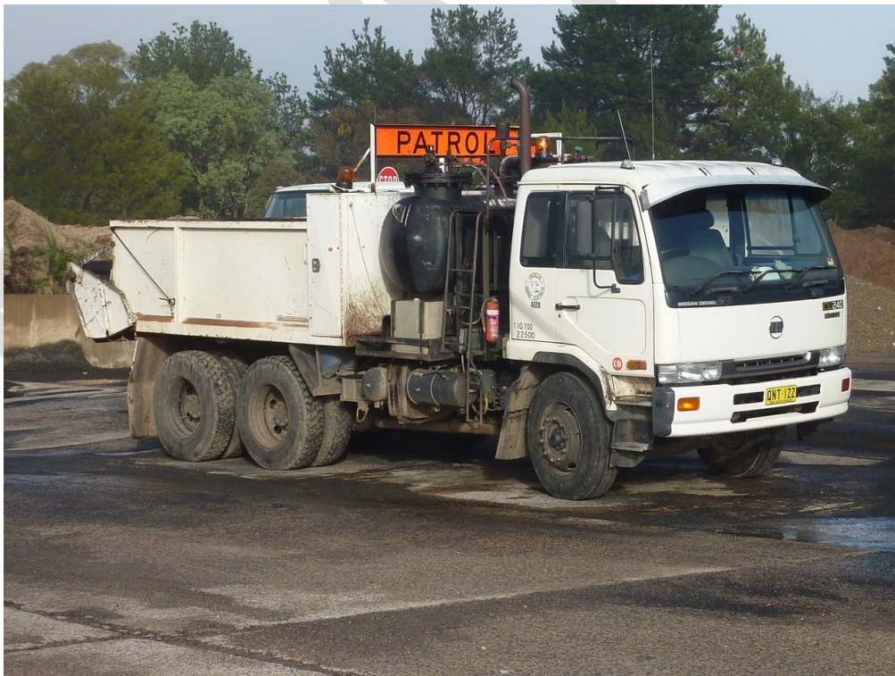
Figure 3 – Council's oldest (26 years) working heavy truck, still serviceable for tar patching operation.
