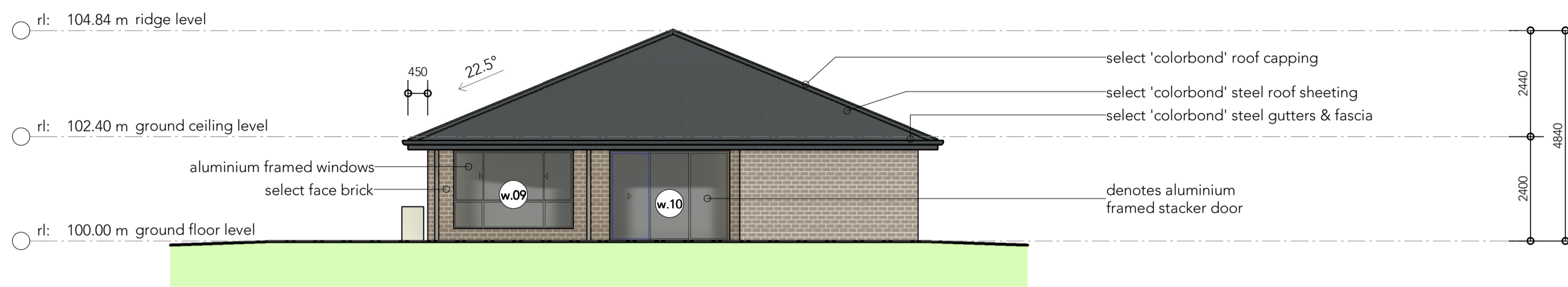
04 elevation: west facade 1: 100 (A1)
