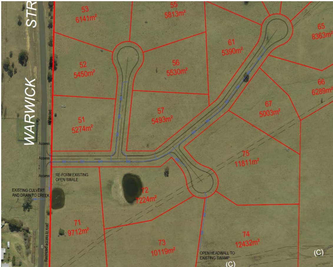
Figure 17.7B Stormwater Servicing Plan
