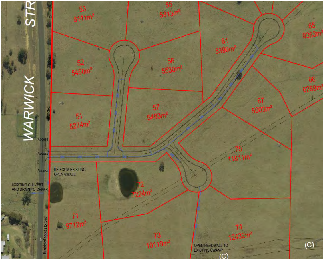
Figure 17.7B Stormwater Servicing Plan
