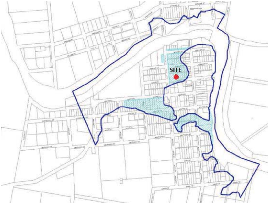
Figure 2: Flood Planning Area at Bundarra. Flood storage areas are hatched in light blue.
