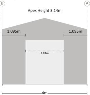
Measurements are from the outside of side girts to the inside of component opening size.
