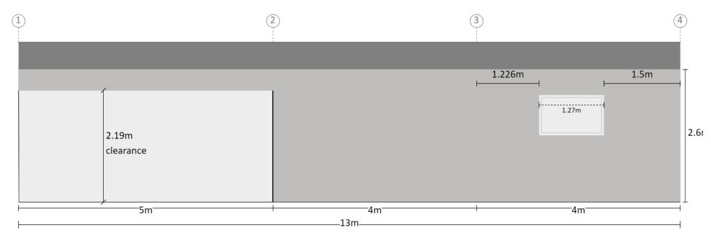
Measurements are from the outside of end girts (end bays) and/or centre of columns (mid bays) to inside of component opening size.
