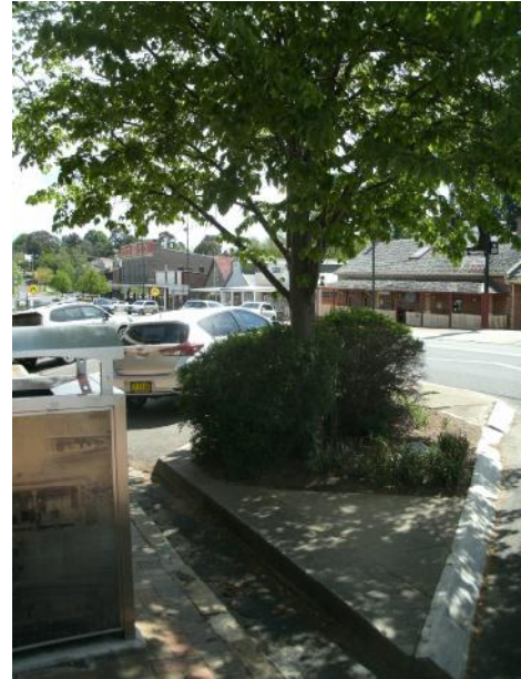
Fig 16 & 17. Street Tree Planting islands encroached by paving and typical existing double kerb drainage with metal plate cover appears like an after thought or solution that does not integrate with the streetscape.
