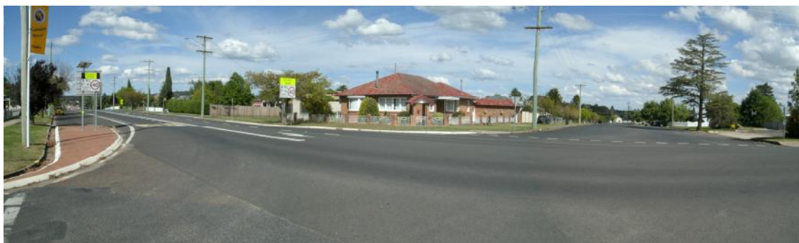
Fig 6. John/Bridge St. 'Traffic Street' intersection: Even with blister for the school Zone sign, there is little enclosure for traffic calming and long distances for pedestrians to cross the Highway.
