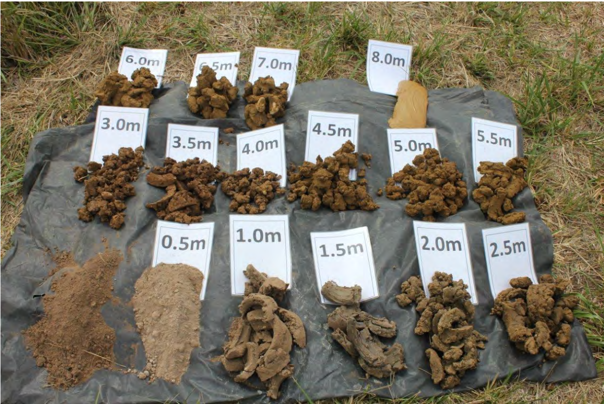
Figure A 1: Auger samples from the test bore
